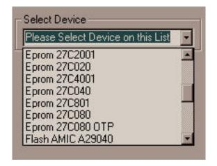
If you select a device that could require programming voltage different from the regular 12.5V, such as 2732 eprom devices, a selection for 21 and 25V will be enable, so you could select the proper programming voltage for that device, as shown below;
